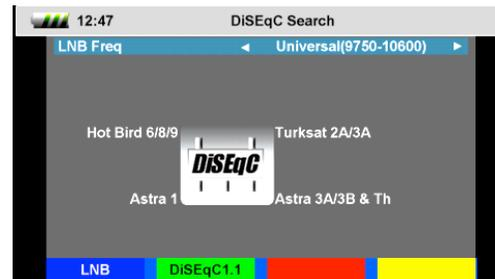
The DiSEqC search begins automatically. In succession, all four DiSEqC1.0 ports are scanned. After completing the scan, the display may look like the image above right.
