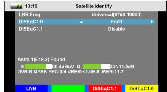
You can see which satellite is currently received on the display screen, as well as the signal strength and quality.
