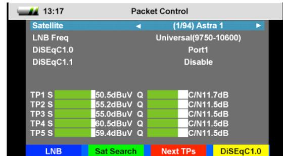
5. If you use a multifeed antenna, go to DiSEqC1.0 and select the port for the selected satellite. You can also change the DiSEqC1.0 port with the yellow FUNCTION key.
